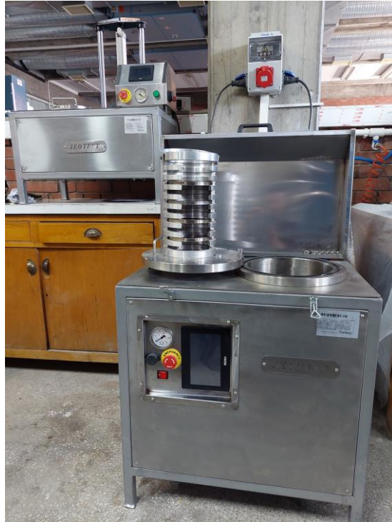
Figure 3.13. Vacuum oven (left) and PAV (right).
