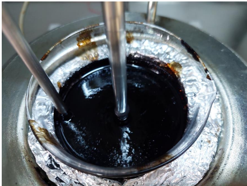
Figure 3.6. Mixing process of the base asphalt and CR.
